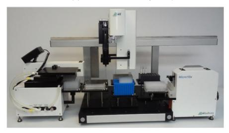
The RapidWash<sup>™</sup> in a Compact, ELISA Workstation with the SOLO automated pipettor and Micro10X reagent dispenser
