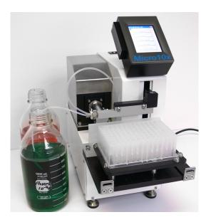
Micro10x<sup>™</sup> - Fast, Compact, Accurate Benchtop Instrument for Reliable & Automated Reagent Dispensing into all Microplates
