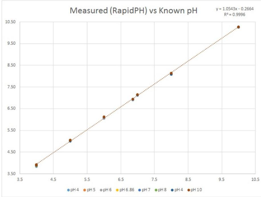
Users who rely on pH measurements are often subject to inconsistent results among manually tested samples. Hudson Robotics' Rapid\_pH™ Automated 96 pH Meter solves this problem by assuring exact consistency of the probe storage, preparation and measurement processes. And, it is FAST!
