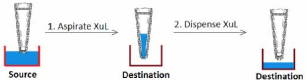
2. **Pre-Aspirate/Blow-Off** – This is the same as Method 1 but is preceded by aspirating a volume of air, followed by a blow-off of the same volume. The blow-off improves the accuracy of this method, but the increased ratio of air/liquid in the system results in reduced precision. This method most closely mimics that achieved with a standard hand-held pipettor.
