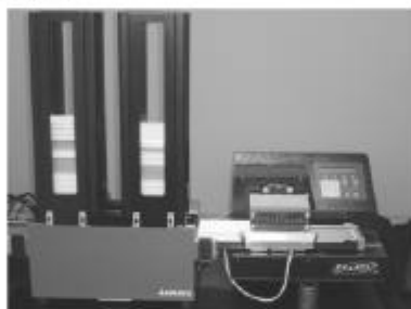
Figure 2: StackLink integrated "online" with Bio-Tek ELx405 Washer.
