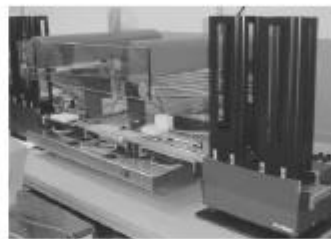
Figure 3: LabLinX integrated with Sias Xertus liquid handler. 3 stop positions are configured on the conveyor, which spans the liquid handler deck and connects 2 StackLinks.
