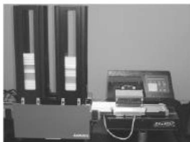
Figure 2: StackLink integrated "online" with Bio-Tek ELx405 Washer.
