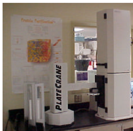
Figure 1. LEADseeker Homogenous Imaging Workstation integrated with a Hudson PlateCrane XT for plate delivery.
