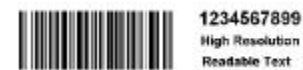
Figure 4: Typical bar code for a microplate label. 3 lines of human readable text are placed to the right of the actual Code 128 bar code.
