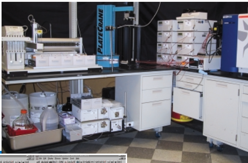
■ The Multiplexed high-throughput HPLC system occupies minimal lab bench space. From left is the Gilson 215 liquid handler, Hudson PlateCrane, Shimadzu UV-Vis detectors, and Micromass LCT-TOF. The Gilson 306 pumps are below the Gilson 215.
