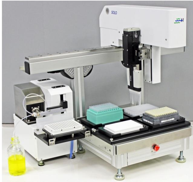
The Micro10x is a small, dependable tool for quickly adding all types of liquids evenly across standard microplates. When connected to the Hudson SOLO robotic pipettor, which can add different test compounds into each well, virtually any assay can be prepared.
