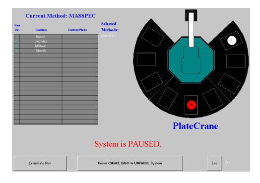
Once a method has been written and stored, it is initiated by selecting F1 Run Method from the Main Menu. The Status Screen shown here will monitor the operations as the plates are moved from the PlateCrane to the HPLC-MS system for analysis.
