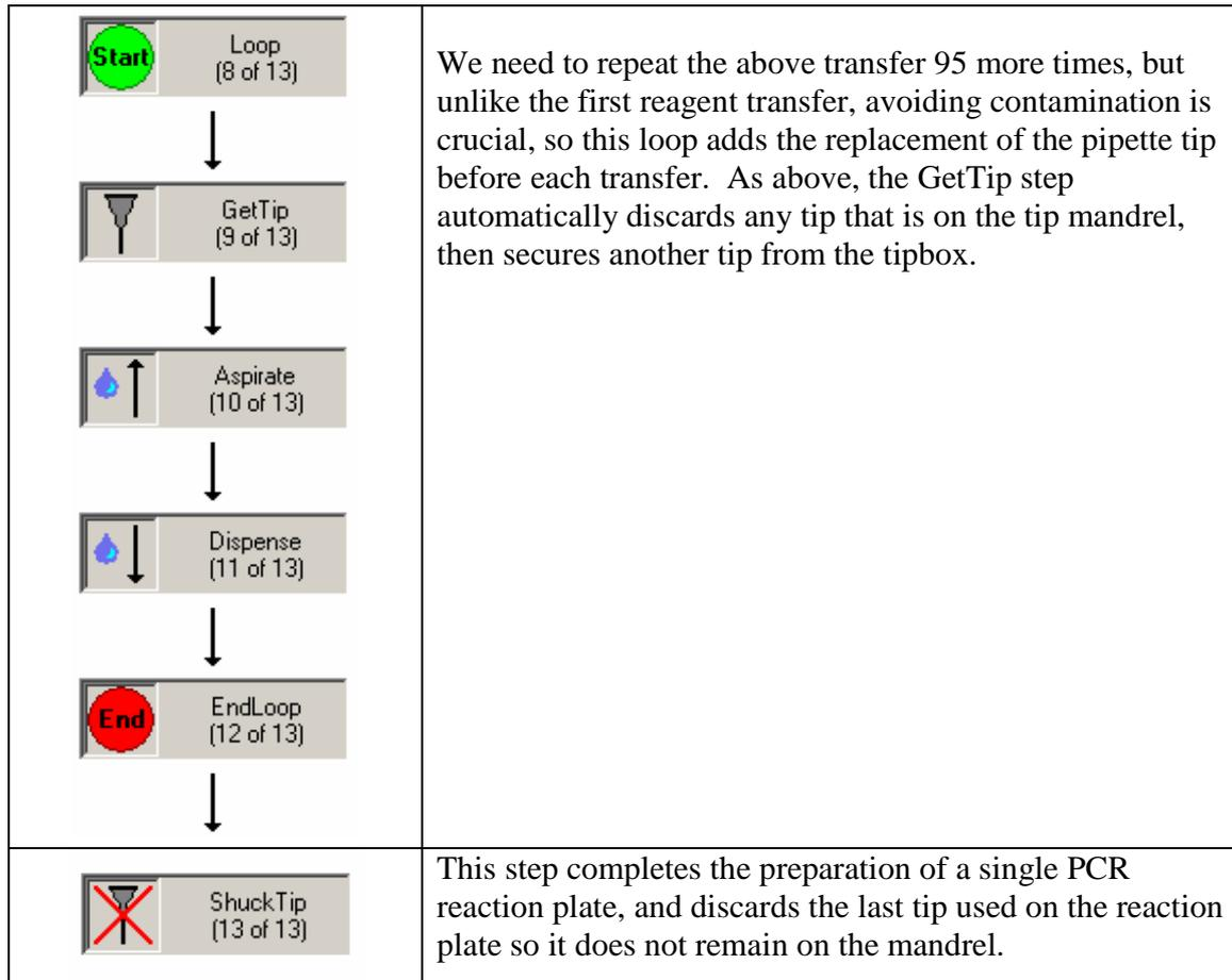
The PCR reaction plate can now be removed from the SOLO and is ready, after sealing, for the thermocycler.
